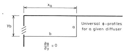
Boundary conditions located close to the constant velocity core of a jet.
