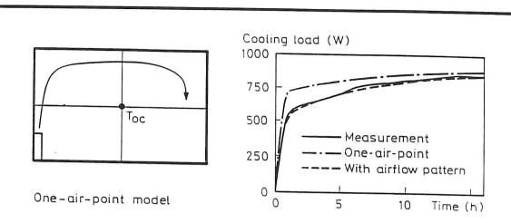
A data base with velocity distribution for different Archimedes' numbers is precalculated and used at each time step in the cooling load programme and temperature distribution is obtained from a solution of the energy equation.
