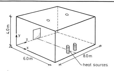
The predictions are made with wall functions, adiabatic boundaries and a radiative energy transfer model.
