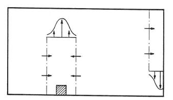
Certain areas can be described by flow elements (thermal flow over a heat source, cold downdraft, concentration distribution around a person, etc.).
